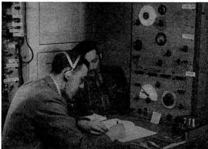
Antenna wizard Dud Charman, G6CJ, at the controls of a massive home-built receiver in the 'thirties. The receiver is believed to have been one of the very first communication receivers built in the UK that included a crystal-gate filter
